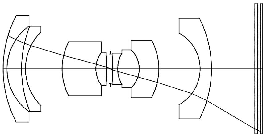
903SWC Biogon 38 with a digital sensor 36x48 mm
